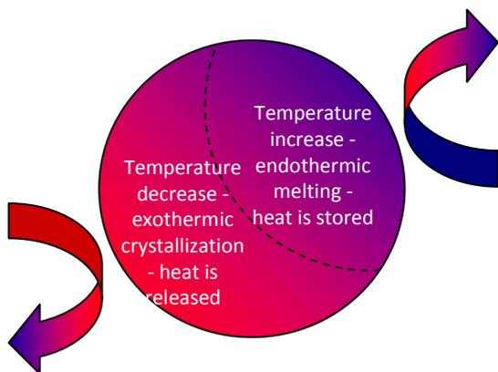
Figure 1 – Principle of a phase change material
